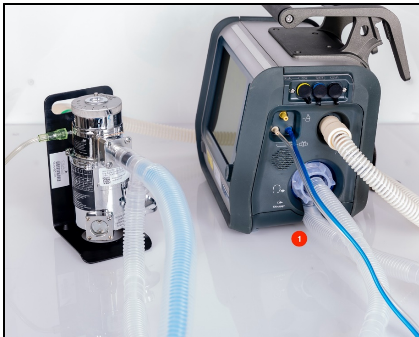
Figure 25. Side view of complete setup of HAMILTON T-1 with UPAC. 1) Bend and kinking of the scavenger tubing
