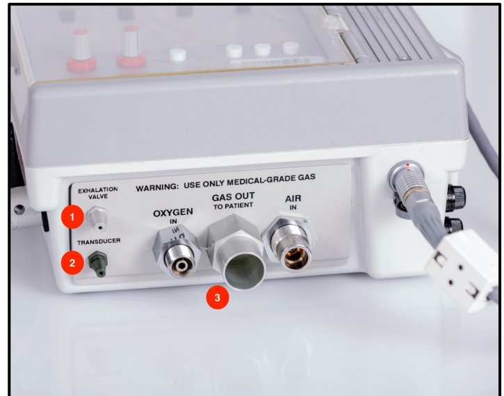
Figure 7. Top view of Impact 754. 1) Attachment for standard circuit expiratory check valve 2) Attachment for standard circuit pressure transducer 3) Attachment for UPAC patient circuit tubing from the basic set
