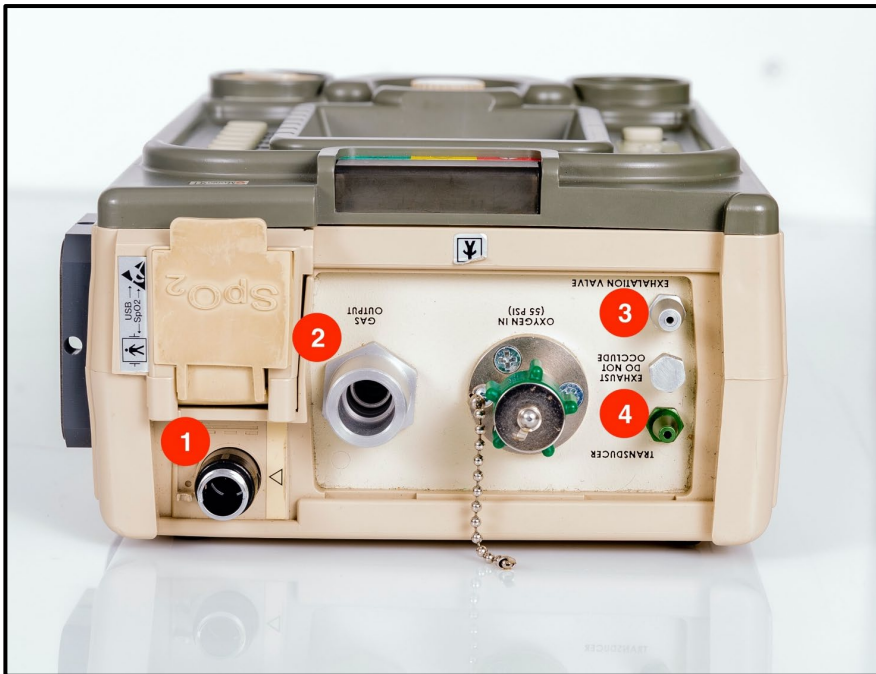
Figure 13. Top view of patient connections for Impact 731. 1) Power connection 2) Attachment for UPAC patient circuit tubing from the basic set 3) Attachment for standard circuit expiratory check valve 4) Attachment for standard circuit pressure transducer
