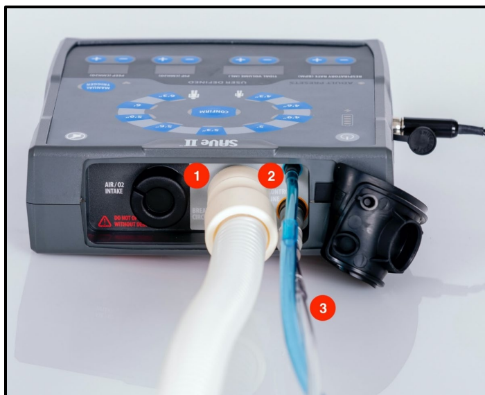
Figure 29. Top view of patient connections for SAVE II. 1) Outlet connection to UPAC via UPAC patient circuit tubing from the basic set 2) Pressure transducer tubing (blue) 3) Expiratory check valve tubing (clear)
