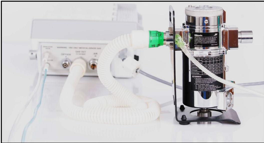
Figure 9. Connection of UPAC patient circuit tubing from the attachment for UPAC patient circuit tubing from the basic set to the vaporizer inlet (Figure 4-1)
