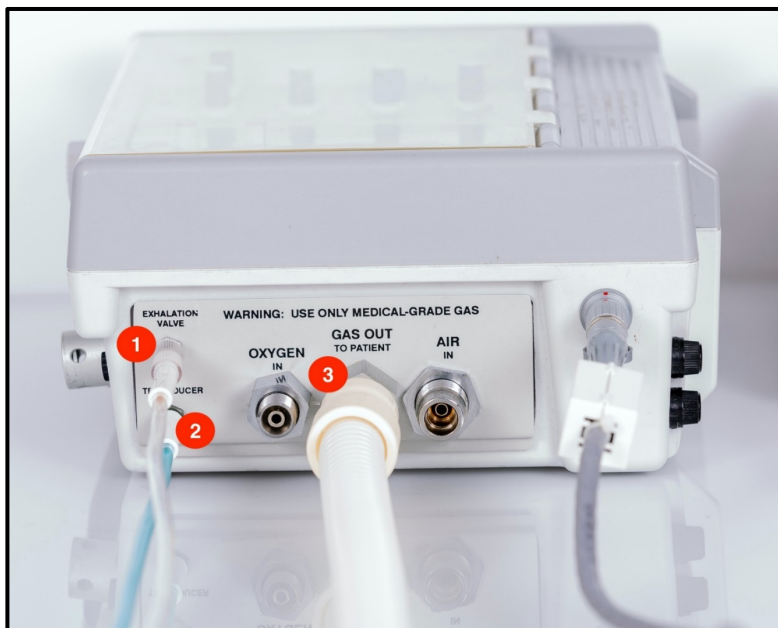
Figure 8. Top view of patient connections for Impact 754. 1) Expiratory check valve tubing connected (clear tubing) 2) Pressure transducer tubing connected (blue tubing) 3) UPAC patient circuit tubing from the basic set
