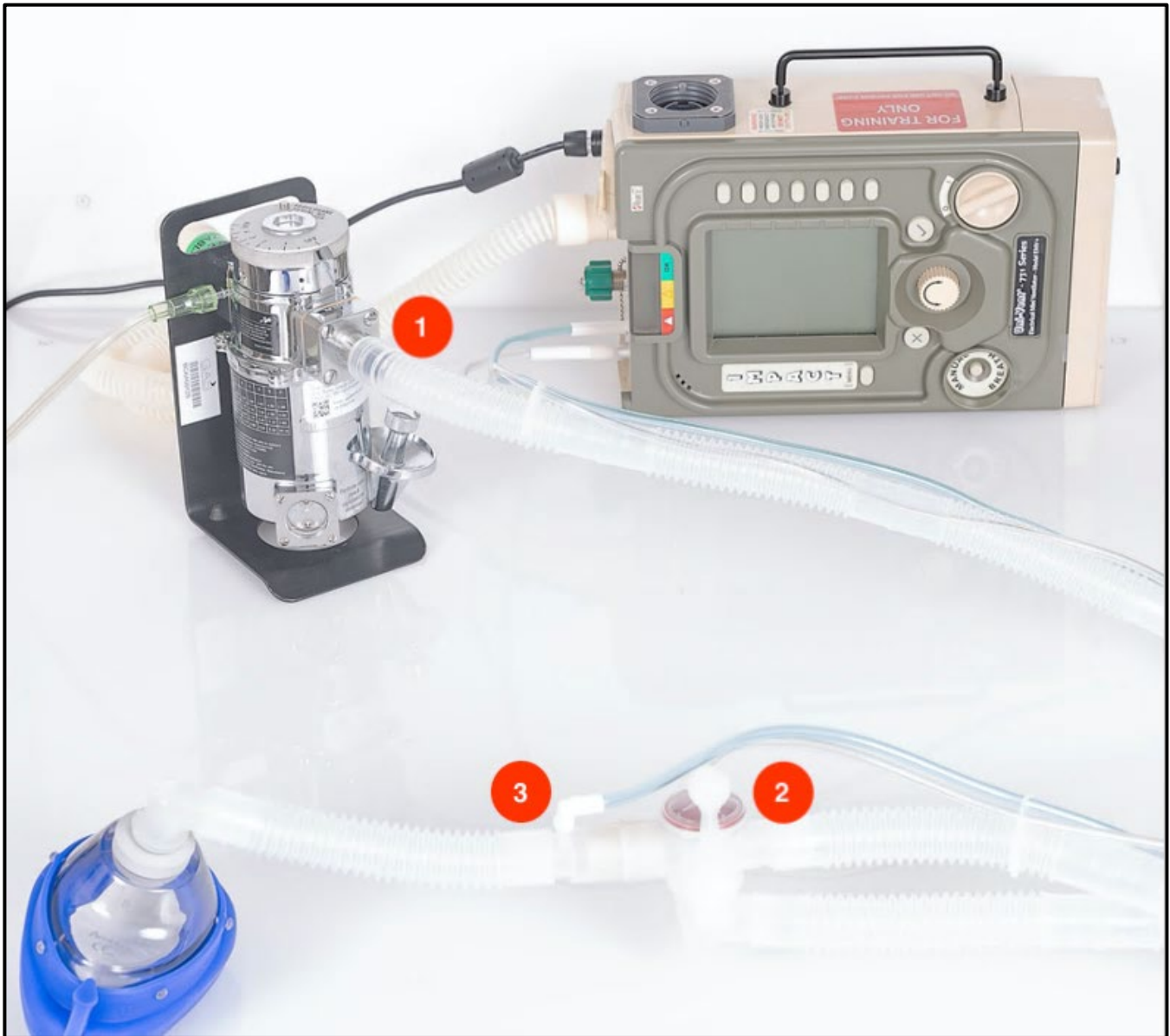
Figure 17. Complete setup of Impact 731 with UPAC. 1) Impact 731 circuit connected to UPAC outlet 2) Expiratory check valve 3) Pressure transducer
