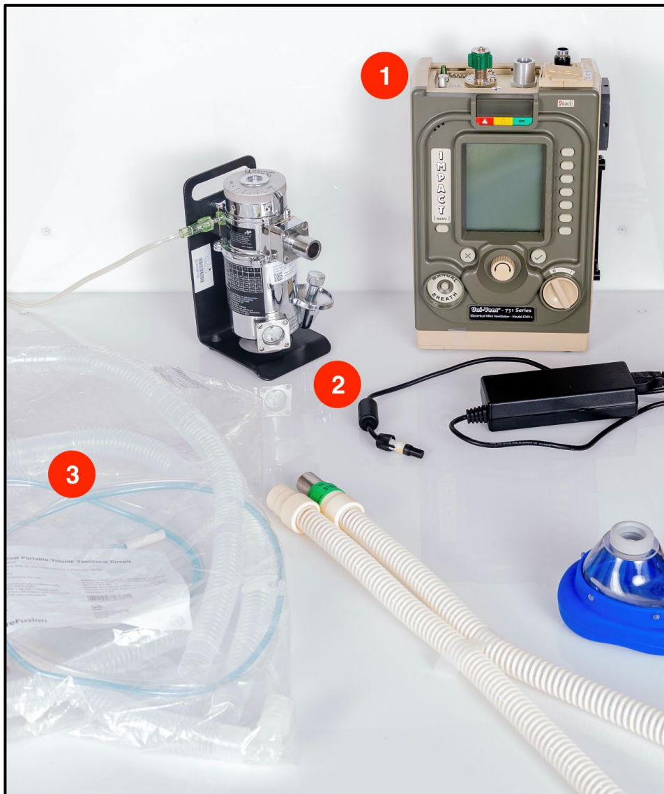
Figure 12. Impact 731 ventilator. 1) Impact 731 2) Power cord 3) Standard Impact patient circuit and UPAC basic set
