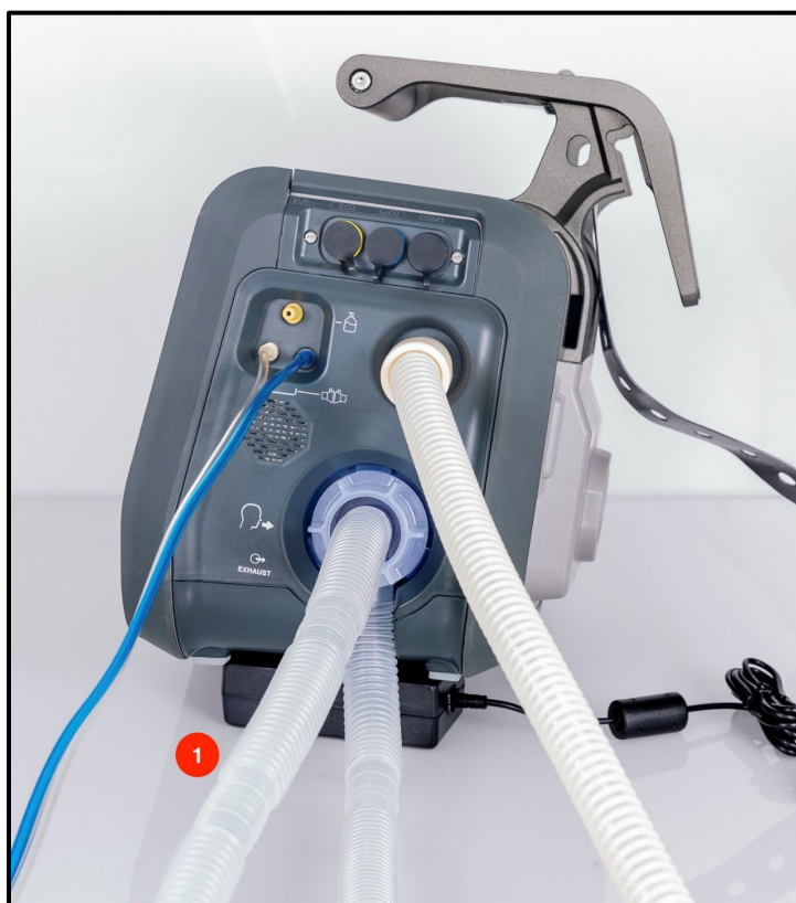
Figure 22. Side view of patient connections for HAMILTON T-1 with expiratory tubing from HAMILTON T-1 standard breathing circuit to ventilatory expiratory check valve. 1) HAMILTON-T1 expiratory tubing
